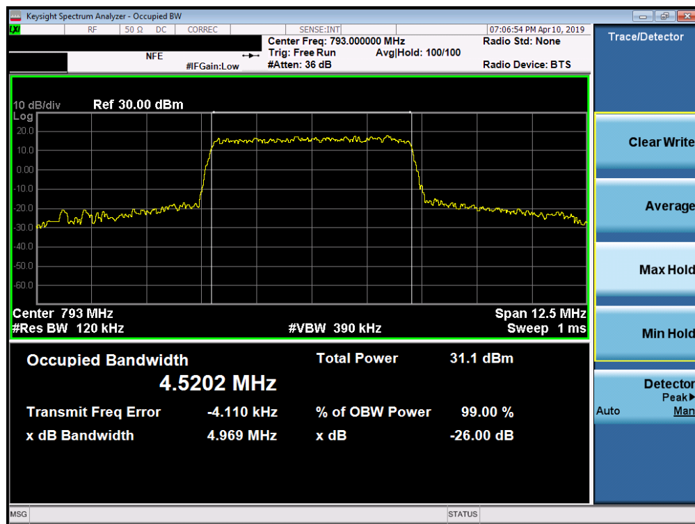
Plot 7-1. Occupied Bandwidth Plot (LTE Band 14, 5MHz QPSK – RB Size 25)
