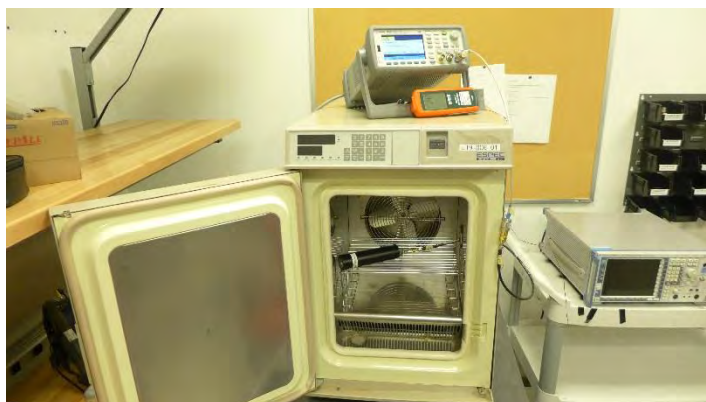
Figure D-1 - Test Setup for Frequency Stability
