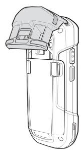
2. Rotate the RFID card reader down, and press down until it snaps into place.
