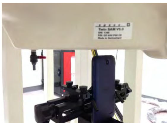
Fig.11 EUT top to flat phantom
