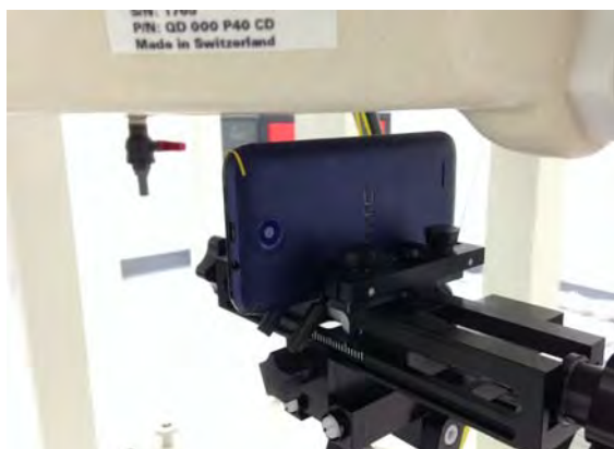
Fig.14 EUT left to flat phantom
