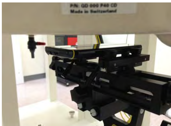
Fig.7 EUT front to flat phantom
