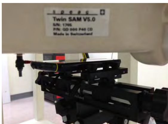
Fig.10 EUT front to flat phantom
