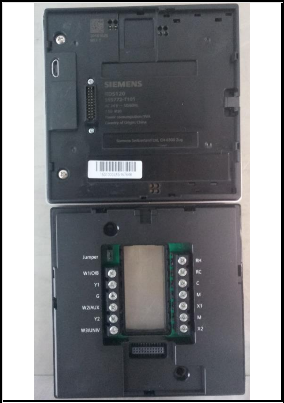
Inside Picture after detaching the HMI module and power module
