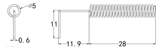
Antenna material : spring steel Antenna wire diameter: 0.6mm Number of antenna coils: 21.4circle
