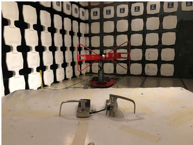
Measurement of Radiated Emission Test Set Up
