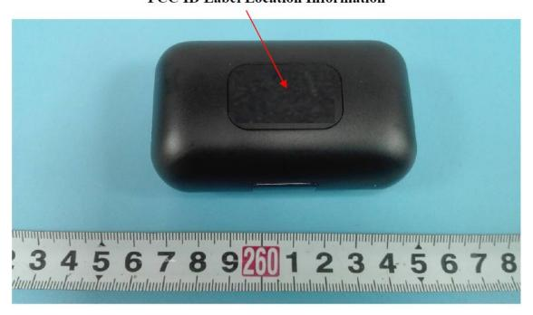
Conclusion: Based on the above description of area A to B, we conclude that the device is unquestionably too small for enabling the FCC ID to be printed onto any surface. We therefore request to move the FCC ID
