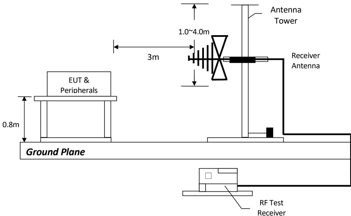
The equipment under test was placed on the top of rotation table 0.8 meter above ground plane.
