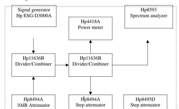
**Processing gain test setup**
