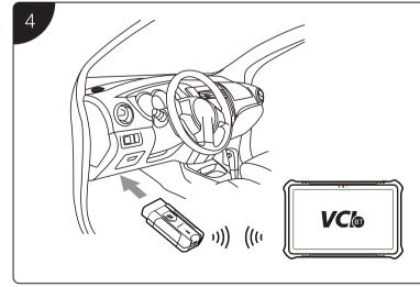
When the V1 is properly connected to the vehicle and the diagnostics tablet, the VCI status button at the bottom bar on the screen displays a green badge. This indicates your diagnostics tablet is ready to start vehicle diagnosis.
