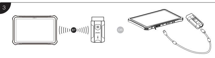
• Pair up the diagnostics tablet with the V1 via Bluetooth to establish a communication link.
