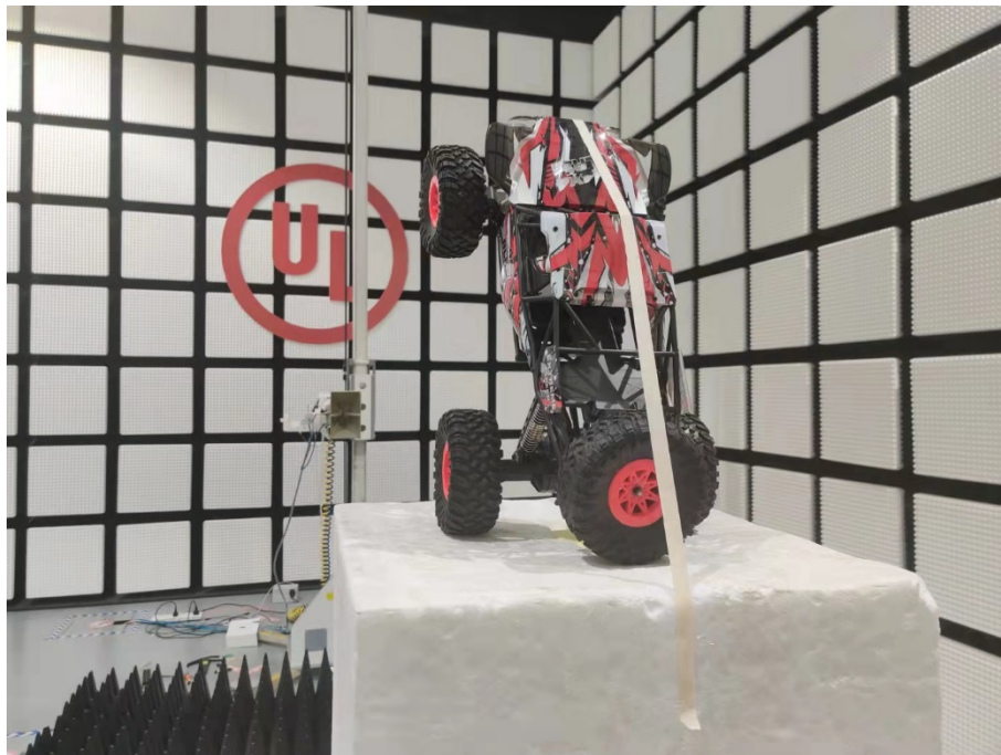
Radiated Disturbance Setup (Above 1 GHz – Z axis)
