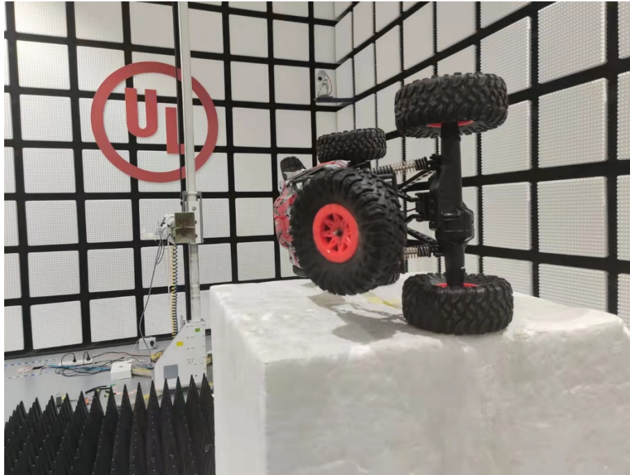
Radiated Disturbance Setup (Above 1 GHz – Y axis)
