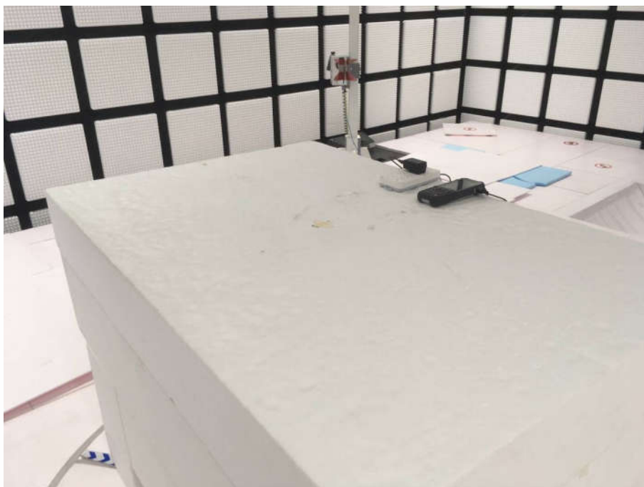
Radiated spurious emission Test Setup-3(Above 1GHz)
