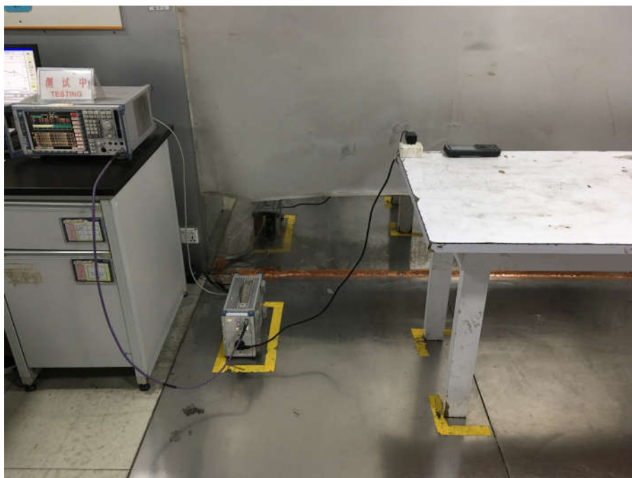
Conducted Emissions Test Setup
