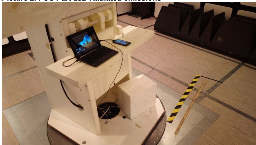
Picture 2. FCC Part 15B Radiated emissions
