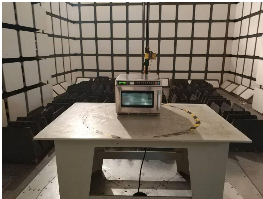
Radiated Emissions - Front View (Above 1 GHz)
