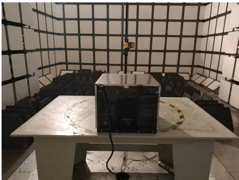
Radiated Emissions - Rear View (Above 1 GHz)
