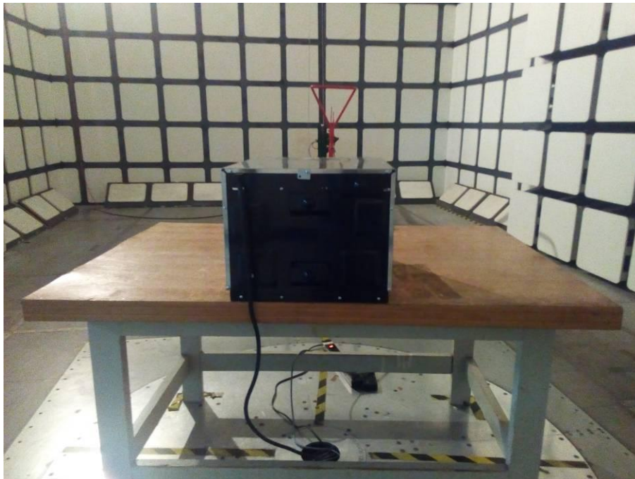
Radiated Emissions - Rear View (30 MHz – 1 GHz)
