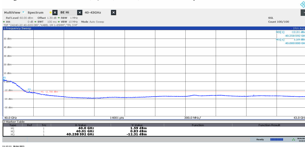
Diagram 2.22c: 40 – 43 GHz, QPSK, TH 8100 , EIRP Horizontal polarization
