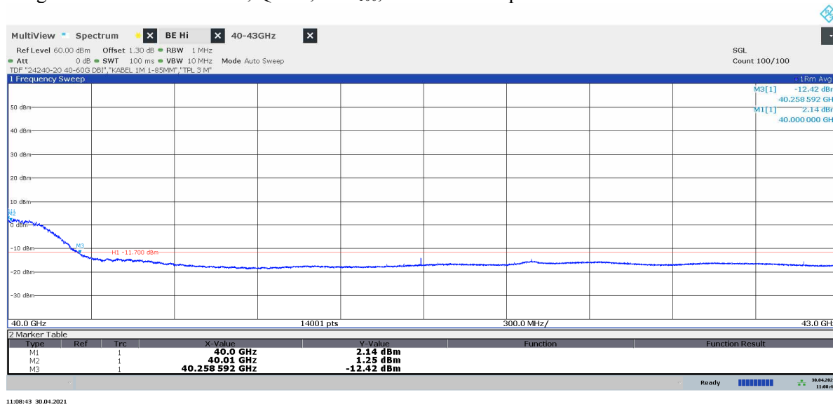
Diagram 2.22d: 40 – 43 GHz, QPSK, TH 8100 , EIRP Vertical polarization
