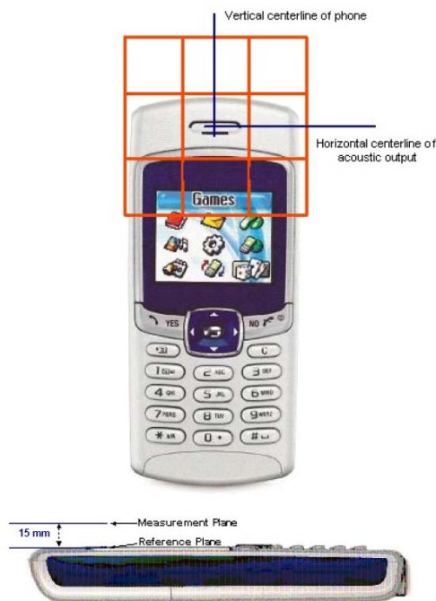
Figure 5.5-2: WD reference plane for RF emission measurement
