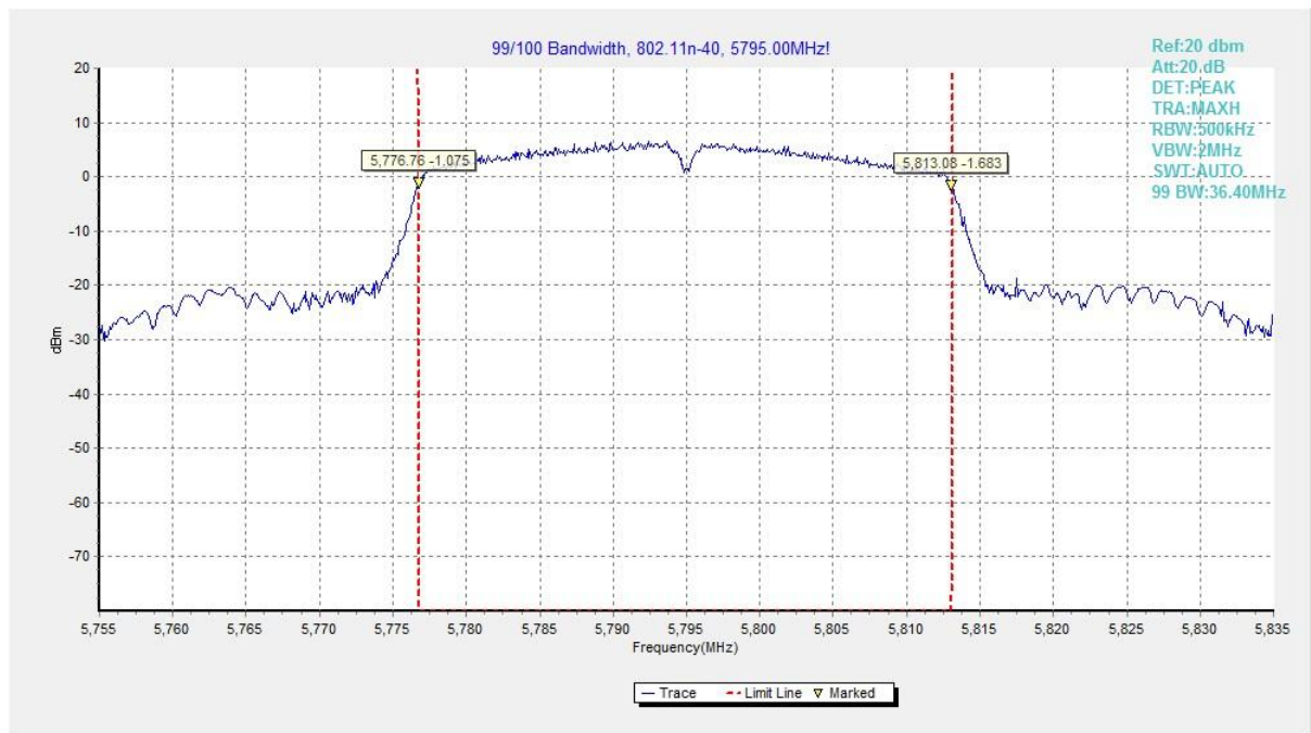
Fig. 33 99% Occupied Bandwidth (802.11n-HT40, 5795MHz)
