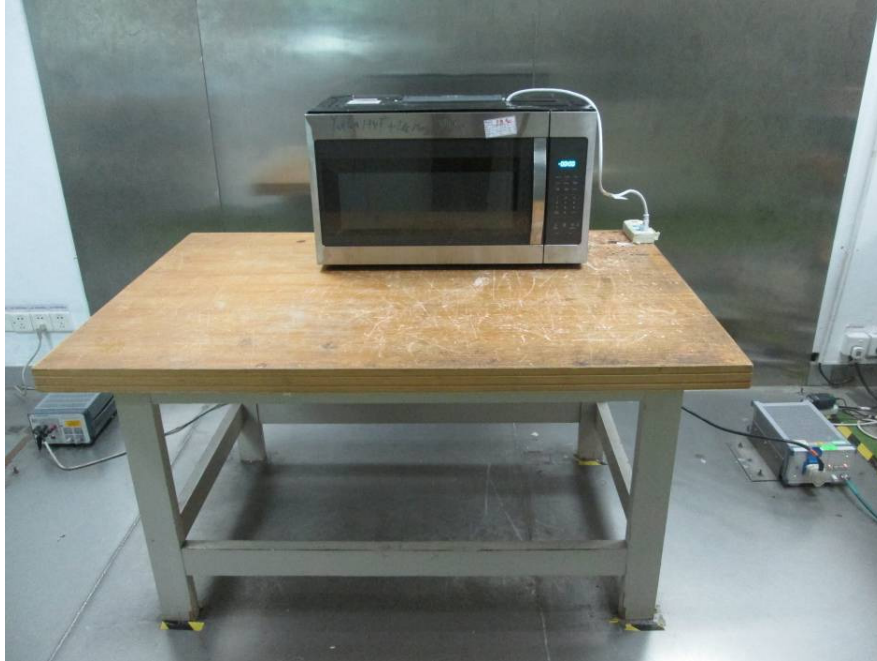
Conducted Emissions - Front View
