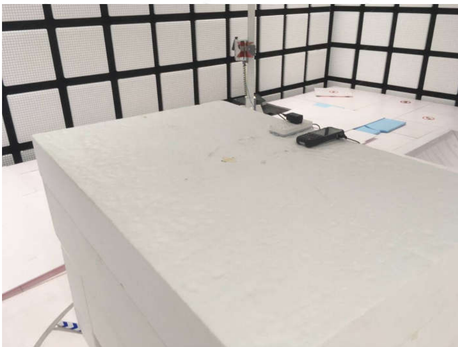
Radiated spurious emission Test Setup-2(Above 1GHz)
