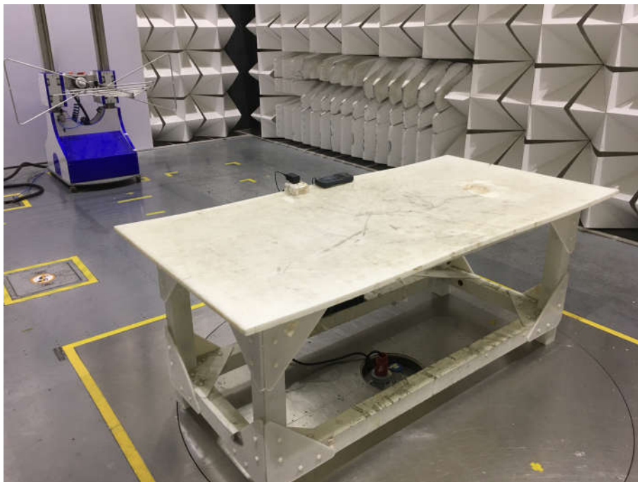
Radiated spurious emission Test Setup-1(Below 1GHz)
