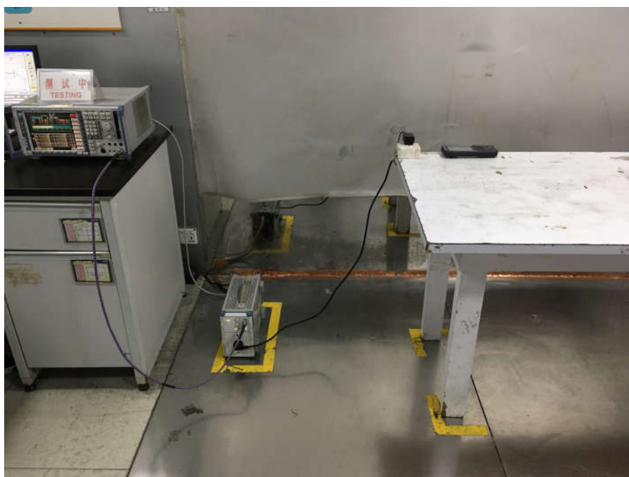
Conducted Emissions Test Setup
