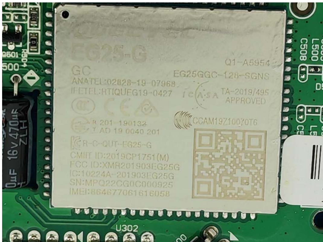
WWAN Module, FCC ID: XMR201903EG25G IC: 10224A-201903EG25G
