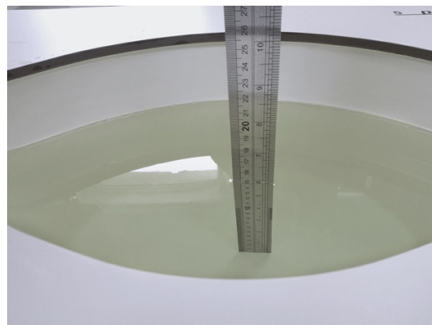
Liquid depth in the body phantom (2450MHz)
