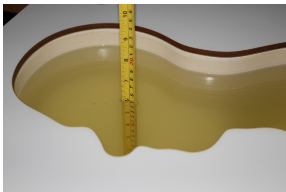
Liquid depth in the head phantom (1750MHz)
