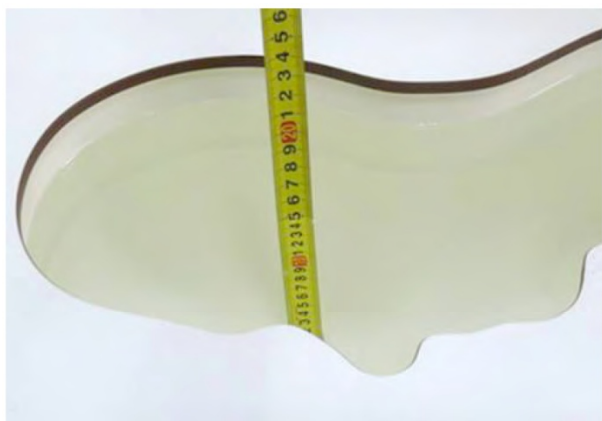
Liquid depth in the head phantom (1900MHz)
