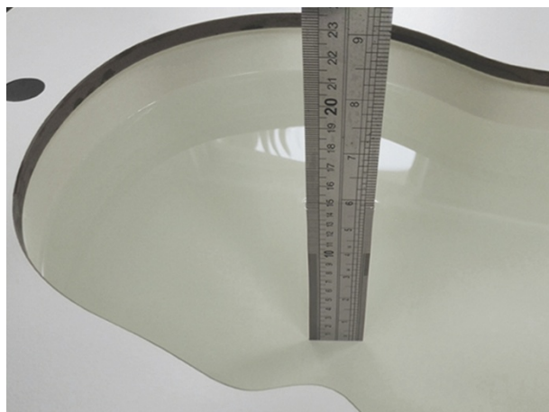
Liquid depth in the head phantom (2450MHz)
