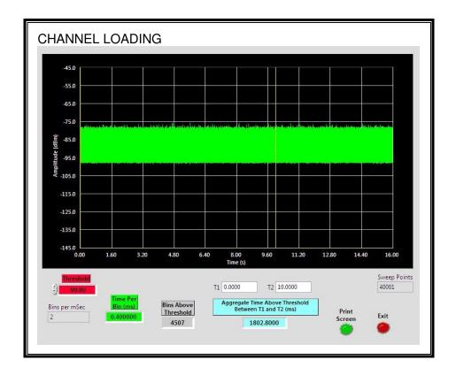
The level of traffic loading on the channel by the EUT is 18.028%
