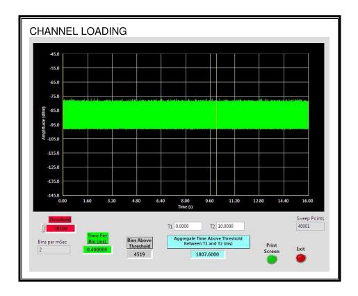
The level of traffic loading on the channel by the EUT is 18.076%
