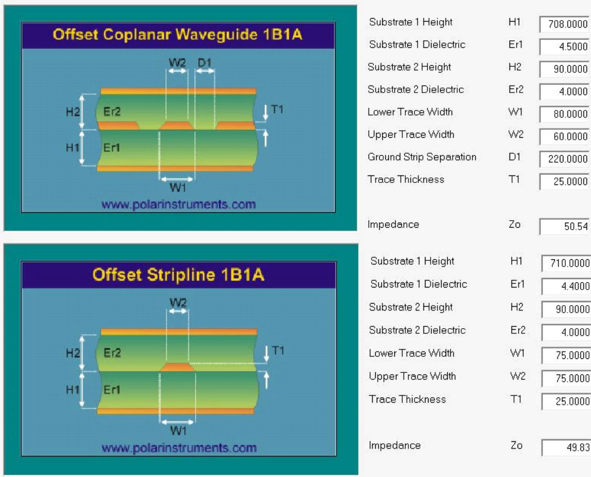
Figure 16: Embedded stripline arrangement example
