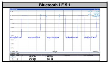
The duty factor of Bluetooth signal has been calculated as following.
