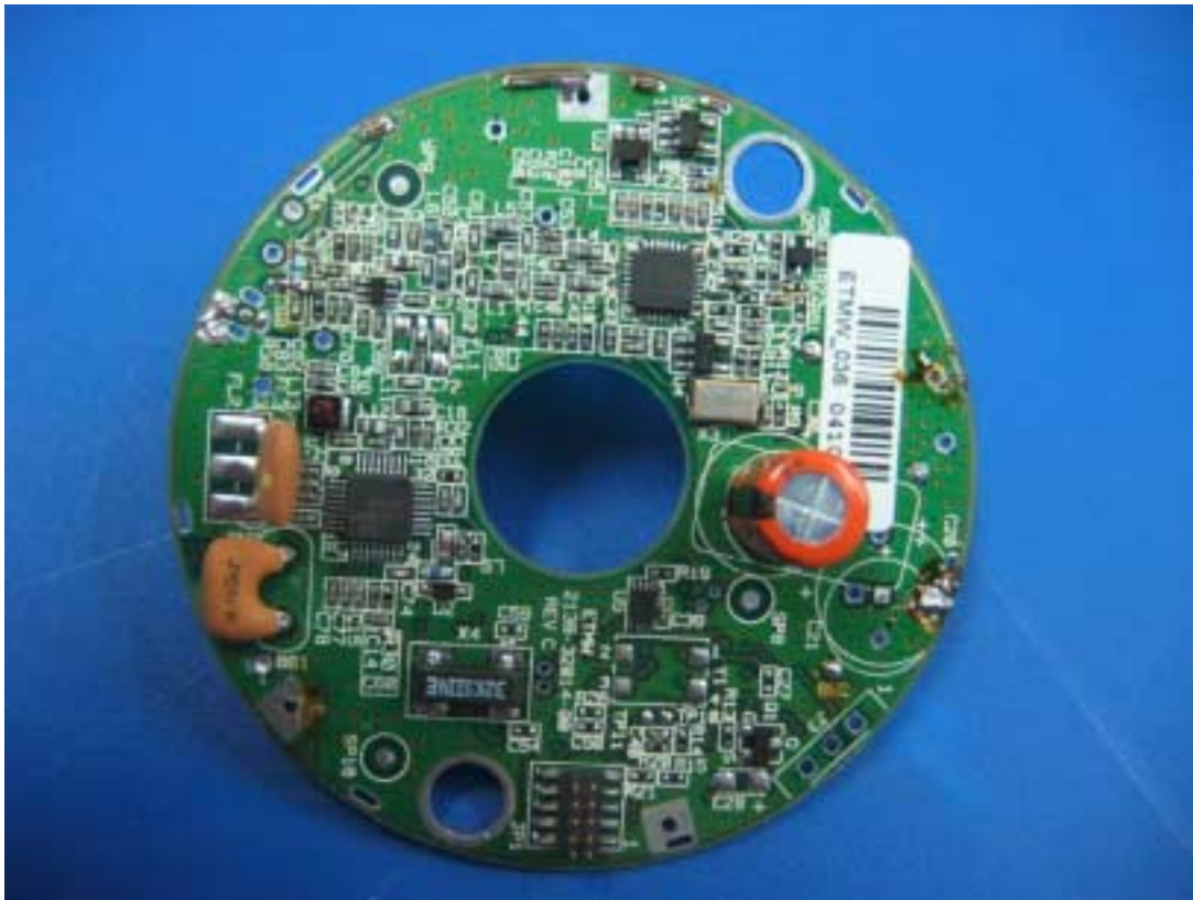
Photograph No.3 ETMW-NA water reader PCB component side without batteries
