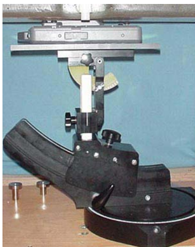
DUT Test Setup with External 2 nd Battery
