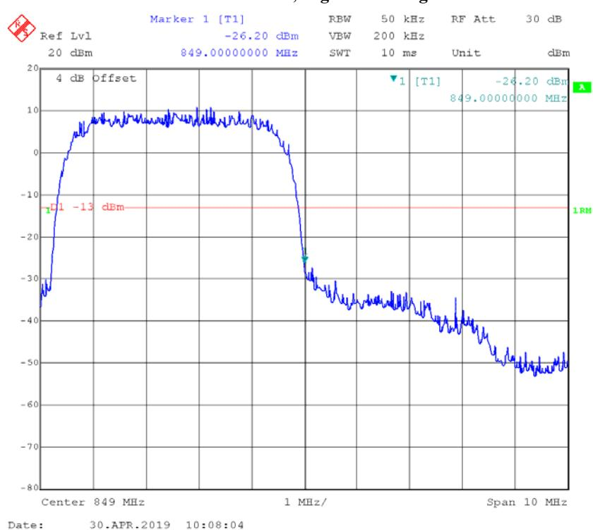
**Band 5 HSUPA, Left Band Edge**
