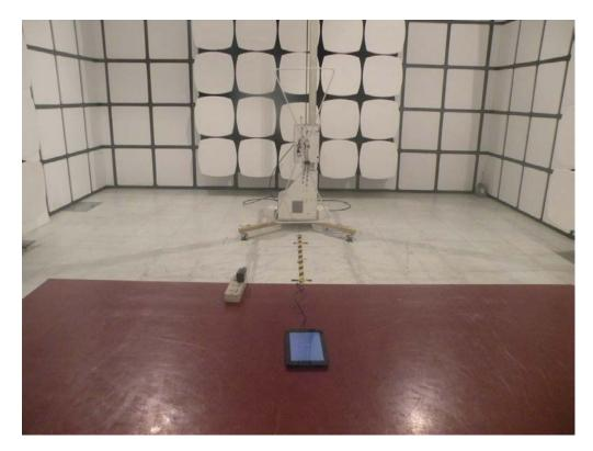
Radiated Emission Test Setup in Chamber
