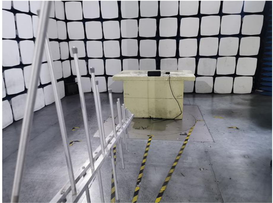
Radiation Emission Test Setup (30MHz to 1GHz)
