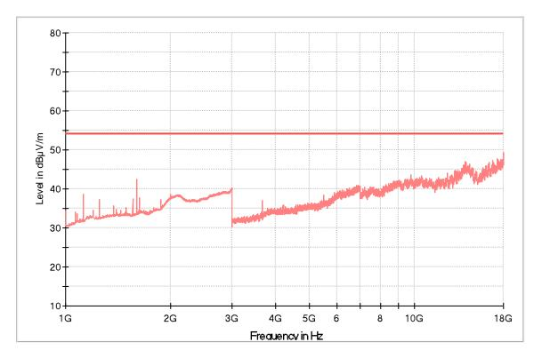
AVG\_MAXH TX limits to Spurious Emission FCC15.249 (Above 1GHz) 902-928MHz\_Average Lim
