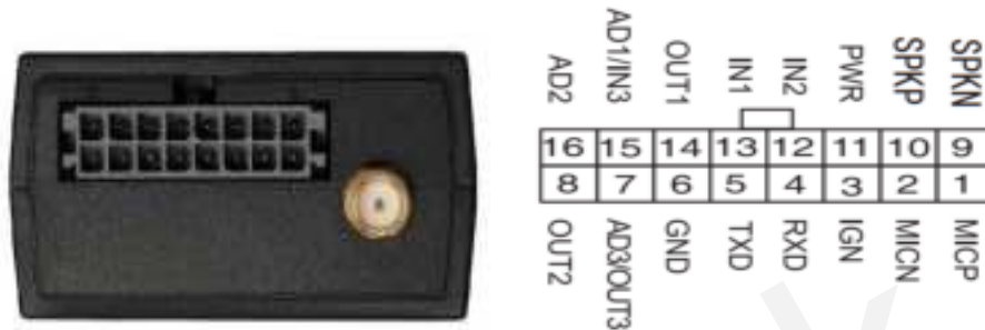
Figure 3. The 16-pin Connector on the GV300LAU
