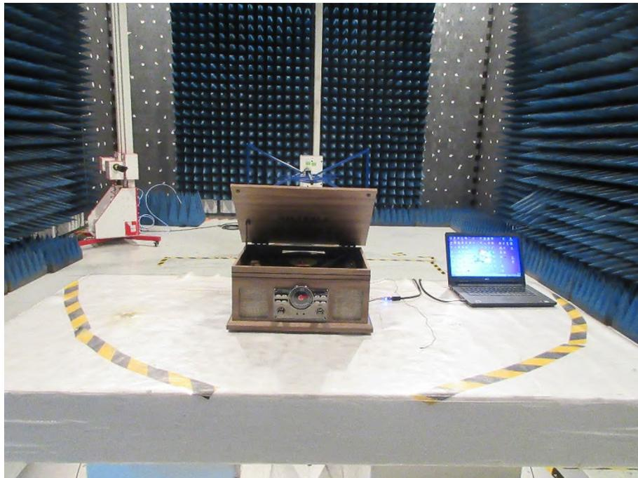
**Photograph 2: Set-up for Radiated Spurious Emission, above 1GHz**
