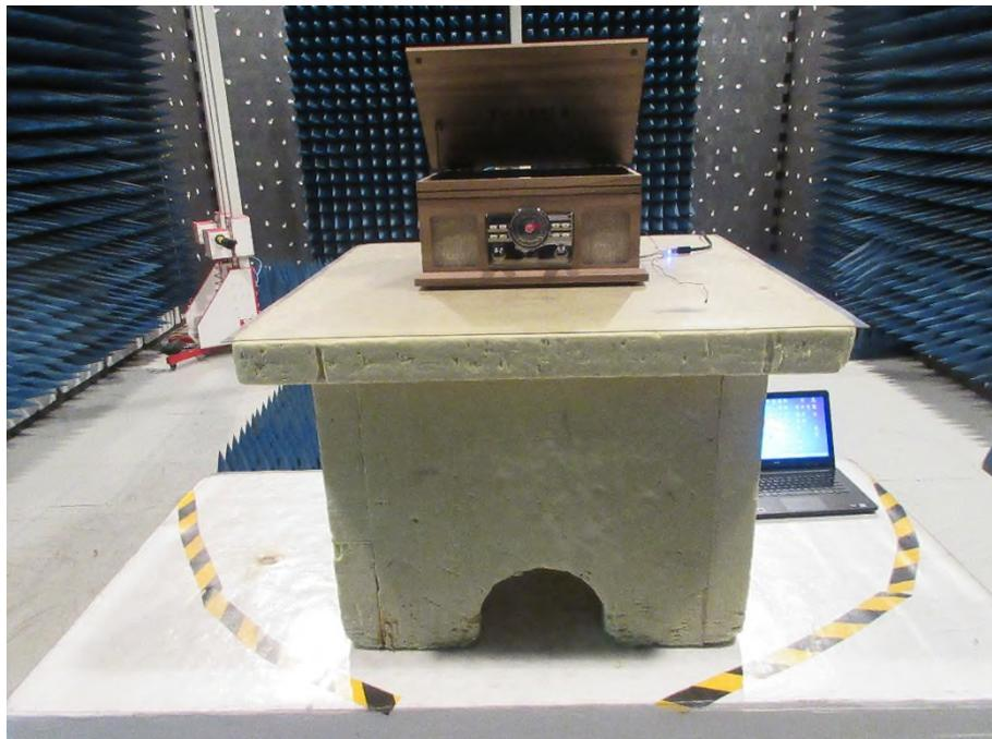
**Photograph 3: Set-up for Conducted Spurious Emission**
