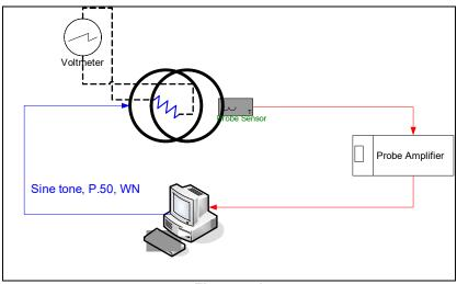
Figure 4-1 Validation Setup with Helmholtz Coil
