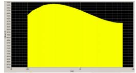
**Figure 4-4** Spectral Characteristic of full P.50
