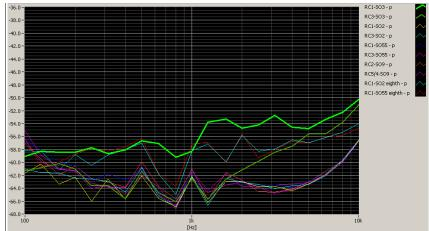
Figure 8-1 CDMA Audio Band Magnetic Noise
