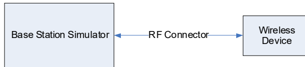
Figure 9-2 Power Measurement Setup
