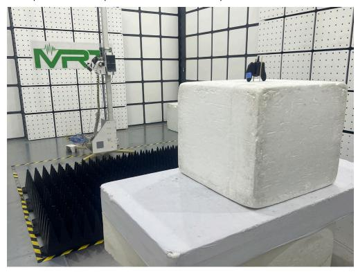
Description: Radiated Spurious Emissions Test Setup for above 18GHz
