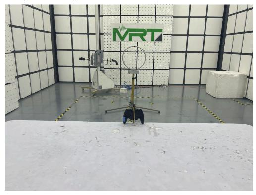
Description: Radiated Spurious Emissions Test Setup for 30MHz ~ 1000MHz
