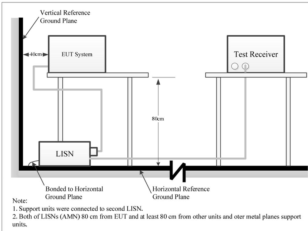
The setup of EUT is according with per ANSI C63.10-2013 measurement procedure. The specification used was with the FCC Part 15.207, RSS-Gen limits.
