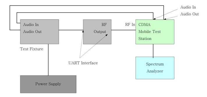
UART Interface: The UART Interface has a serial communication link that can be used to test, debug or upgrade the phone's functions and characteristics.
