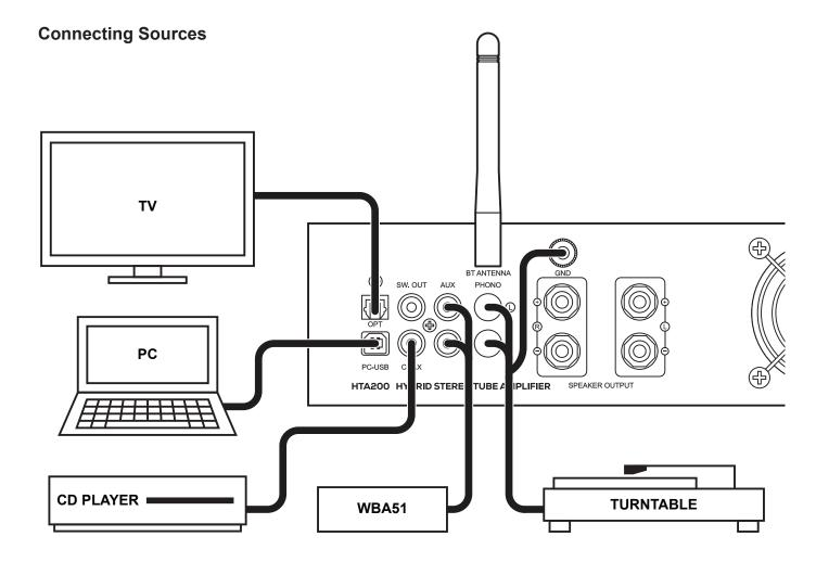
The HTA200 is capable of receiving signals directly from a wide variety of sources. Using high quality cables will ensure the best possible transmission from your connected devices.
