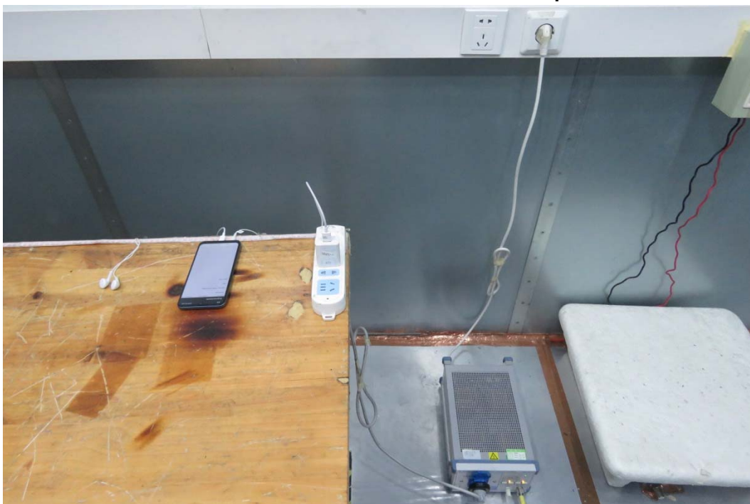
Picture 2 Conducted Emission Test Setup
