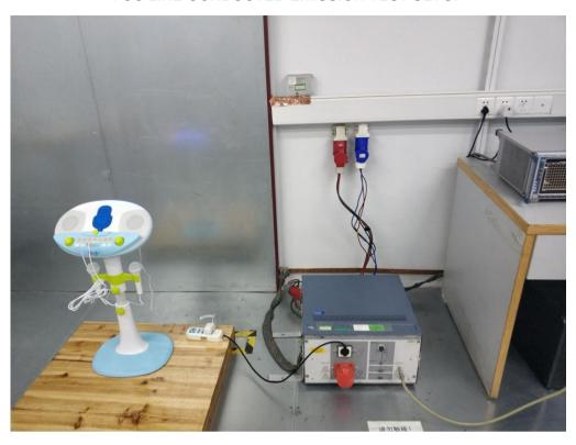
FCC RADIATED EMISSION TEST SETUP
