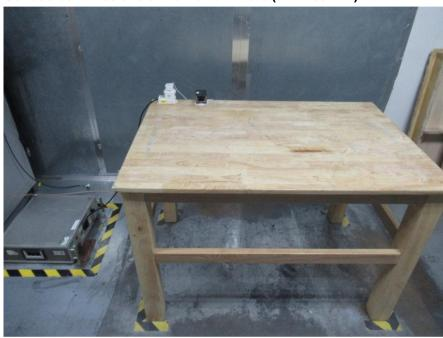
Radiated Emissions (Magnetic field Strength)(9kHz-30MHz)
