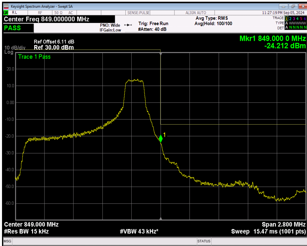
Band5 QPSK BW=1.4MHz Channel=20643 RB Size=6 Position=#0
