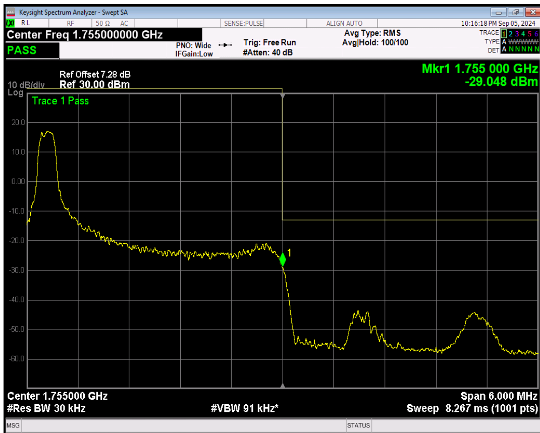
Band4 QPSK BW=3MHz Channel=20385 RB Size=1 Position=#Max
