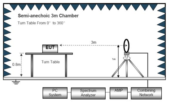
(B) Radiated Emission Test-Up Frequency 30MHz~1GHz
