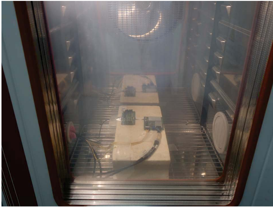
Photograph 3: Set-up for Frequency Tolerance, Inside Temperature Chamber
