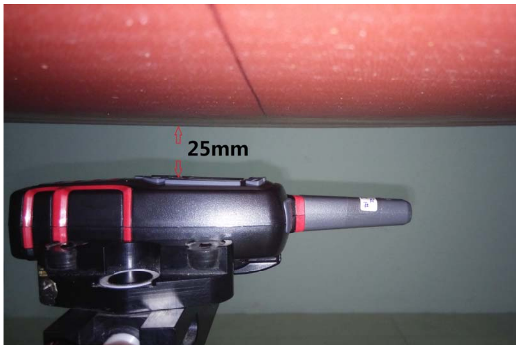
Face-held, the front of the EUT towards phantom (The distance was 25mm)
