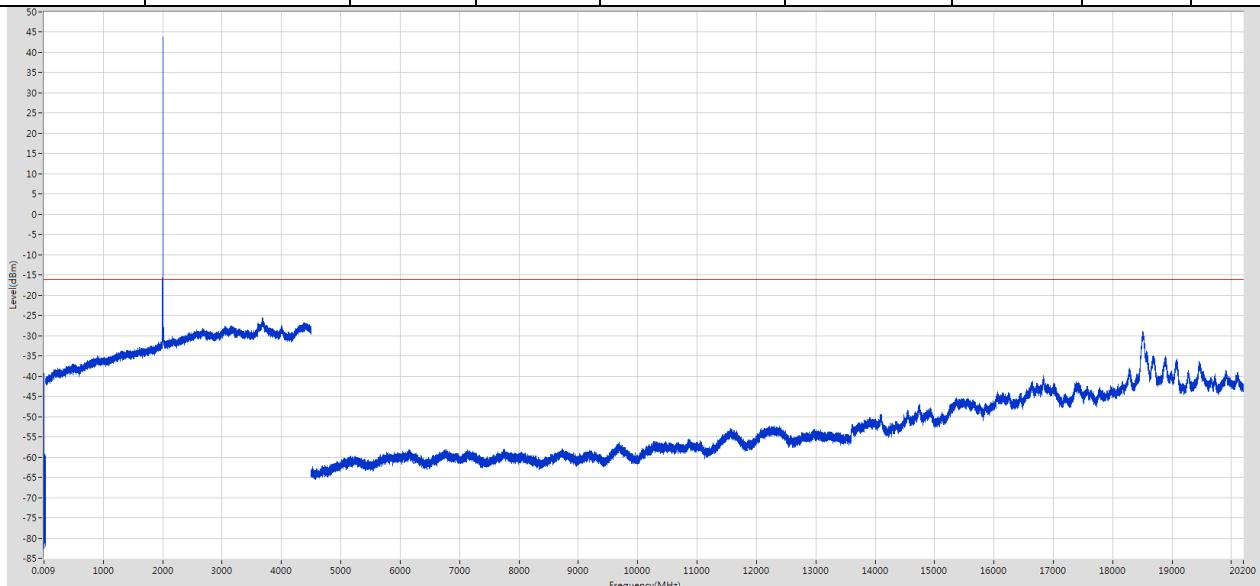
Note: the spike exceeds the limit is the fundamental emission.
