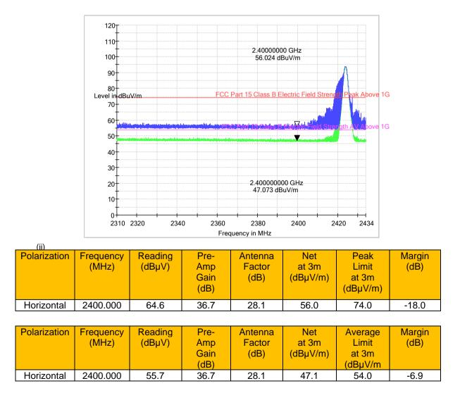
The resultant field strength meets the general radiated emission limit in section 15.209, which does not exceed 74dBµv/m (Peak Limit) and 54dBµv/m (Average Limit).
