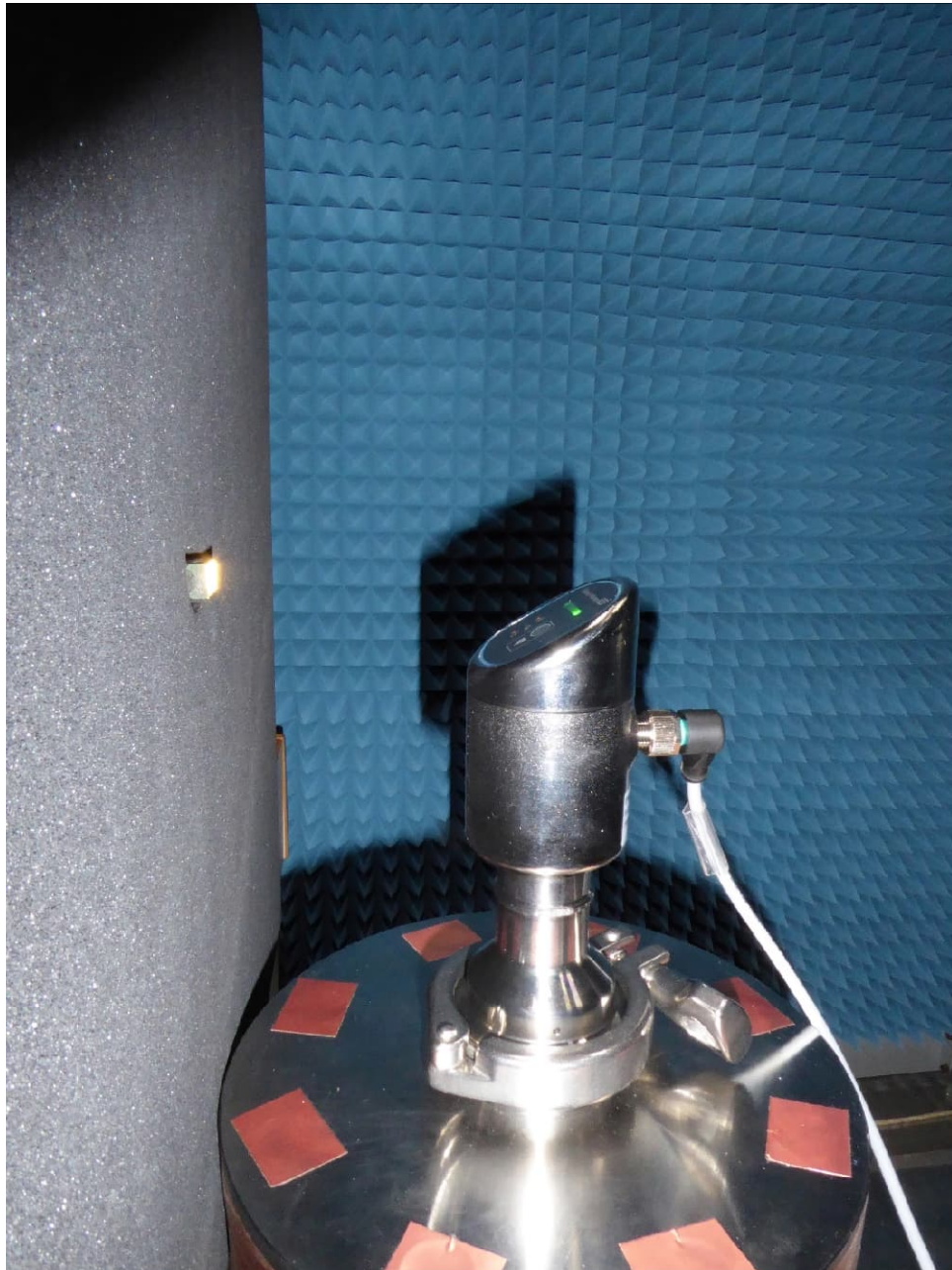
Test setup with EUT 4 (>40 GHz)
