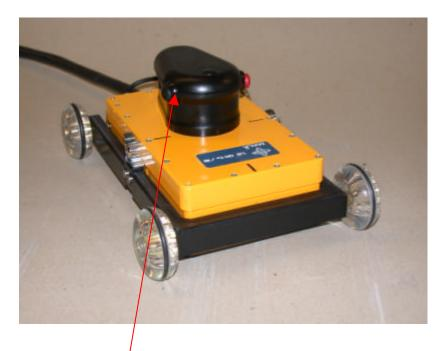
Kill switch, must be constantly depressed. When switch is released, pulse generator will cease firing pulses within 10 seconds.
